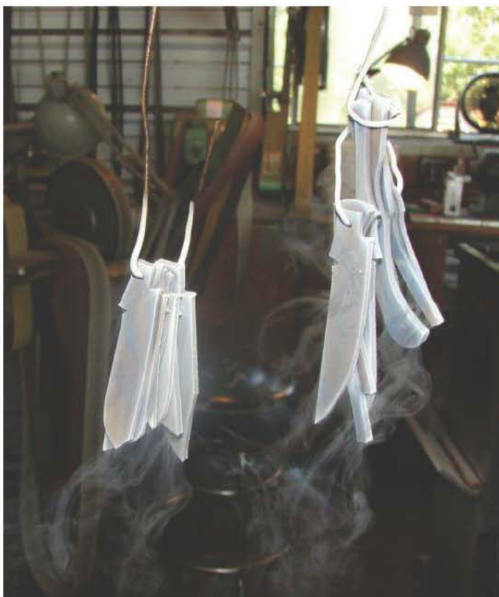
Menefee Made pocketknife blades coming out of the liquid nitrogen cryogenic quench. A cryo quench after heat treatment helps impart more durability.
